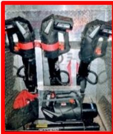
Each powered rescue tool receives its power from the battery power unit component and generates the output forces of energy used to perform one or more of the functions of spreading, lifting, holding, crushing, pulling, or cutting. These tools include cutter, ram(s) and spreader. These rescue tools are not restricted by wires or hydraulic hoses.
