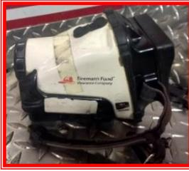
The Department operates four (4) Thermal Imaging Cameras (TIC) and are types of thermographic camera used in emergency services. By rendering infrared radiation as visible light, such cameras allow firefighters to see areas of heat through smoke, darkness, or heat-permeable barriers. Additionally, 14 SCBA have integrated TIC's for firefighters' immediate use in a hazardous environment.
