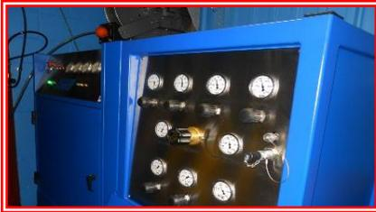
*This unit is 10 years old.* The in-house air compressor has high-pressured capabilities up to 6,000 psi and certified as grade D breathing air as required by the Compressed Gas Association. The unit has a quarterly air sample analysis completed to assure the highest grade of quality breathable air and the proper operation of the unit and to comply with NFPA Standards.
