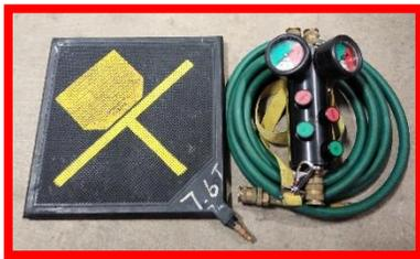
The Department maintains 2 sets of air bag rescue systems capable of lifting 134 tons. Air bags can be used in a variety of incidents including building collapses, heavy extrications and industrial entrapments. Air bags can be adapted for many other situations such as to displace, spread or otherwise move objects.
