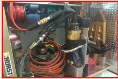
Hydraulic rescue tools are used by emergency rescue personnel to assist in the extrication of victims involved in vehicle accidents, as well as other rescues in small spaces. The Department operates a full complement of powered hydraulic rescue tools on 4 different apparatus to assure availability. These tools include cutter, ram(s) and spreader. Additionally, hand tools, electrical tools and rope rescue equipment are owned and operated by the Department.
